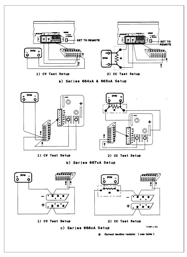
Figure B-1. Verification Test Setup
